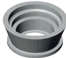
180.X.000050 - HM sleeve For fixing on supporting cross bars at high liquid temperature levels ( > 60^{\circ}\text{C} ) or strong vaporisation at the bottom of the box. Hole diameter: 70 mm - 76 mm. Material: EPDM
